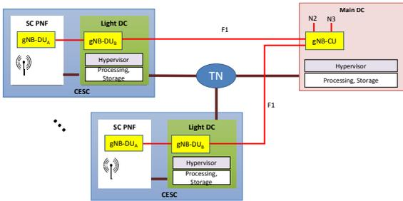
Fig. 1. Example 1: gNB-CU at the Main DC and gNB-DU at the CESC
