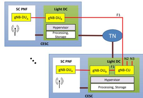
Fig. 4. Example 4: Both gNB-DU and gNB-CU at the Light DC
