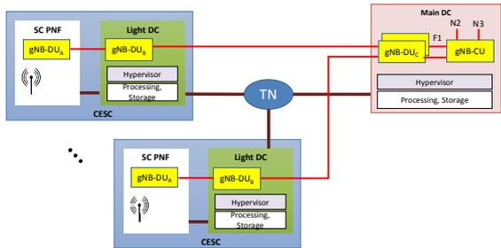
Fig. 2. Example 2: gNB-CU at the Main DC and gNB-DU split between the CESC and the Main DC
