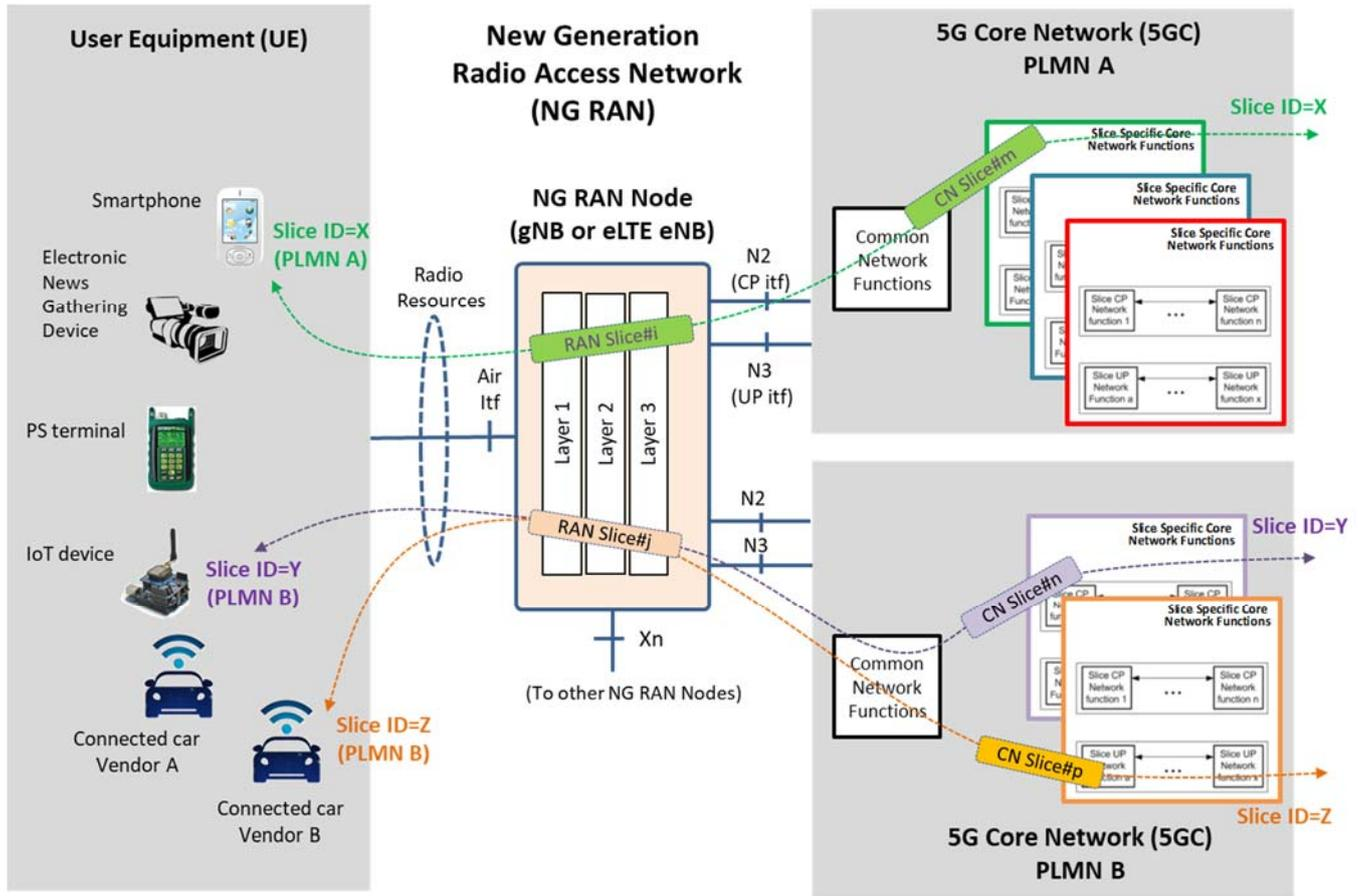
Fig. 1.- Illustration of the network slicing architecture
