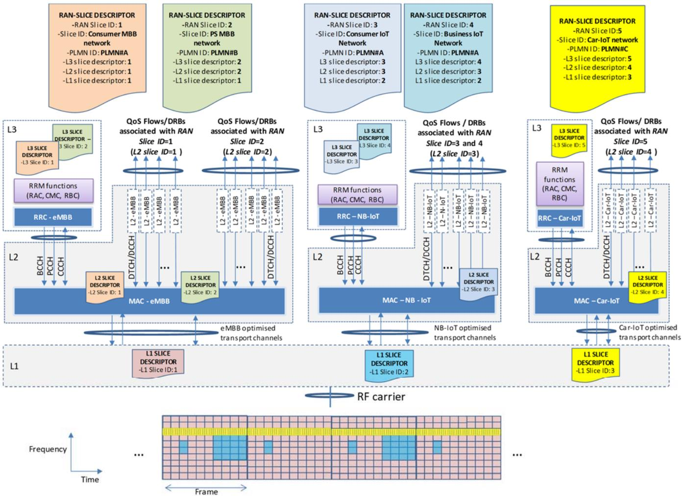
Fig. 4.- Radio protocol stack view of the RAN slicing configuration
