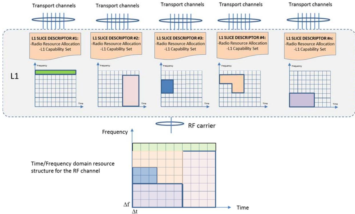
Fig. 3.- Illustration of slicing support in L1
